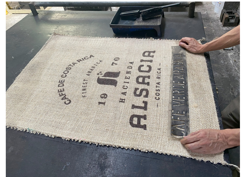
Printing on hessian sacks, prior to filling, using food safe vegetable based inks and templates.
