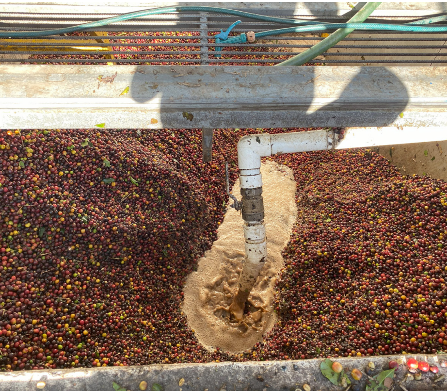
Syrupy water flushing the cherries from the reservoir upwards into the pulper.
