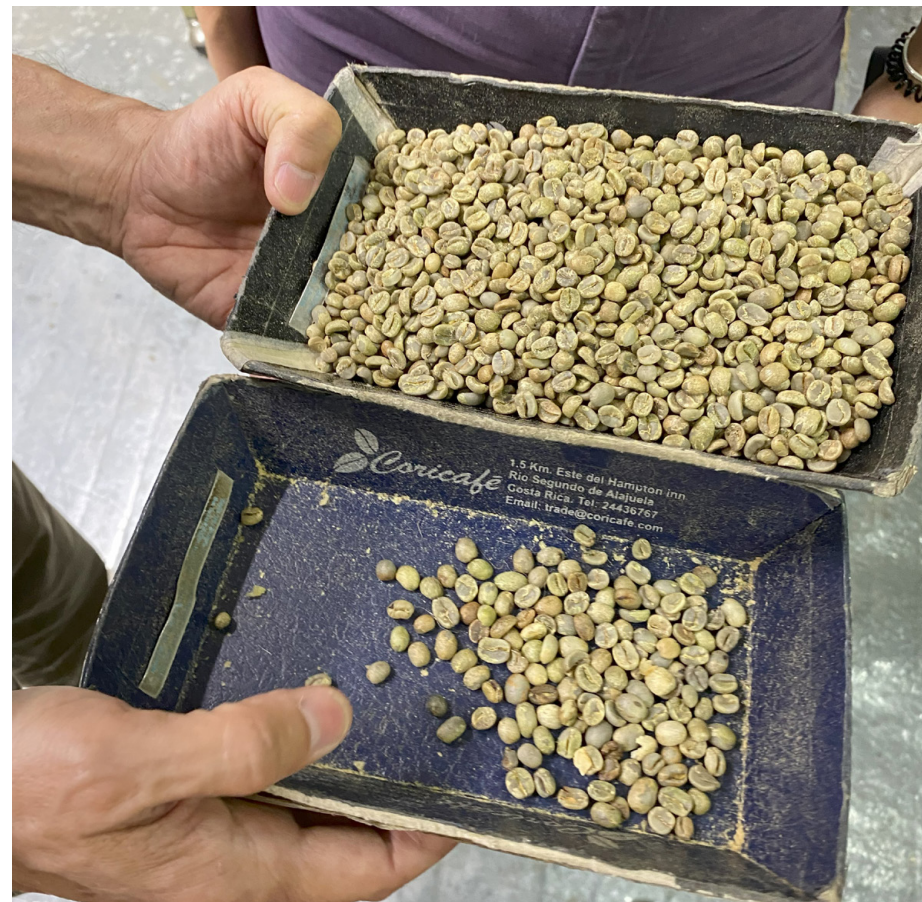
Defects (bottom tray) removed during the dry milling process because of size, colour, damage.
