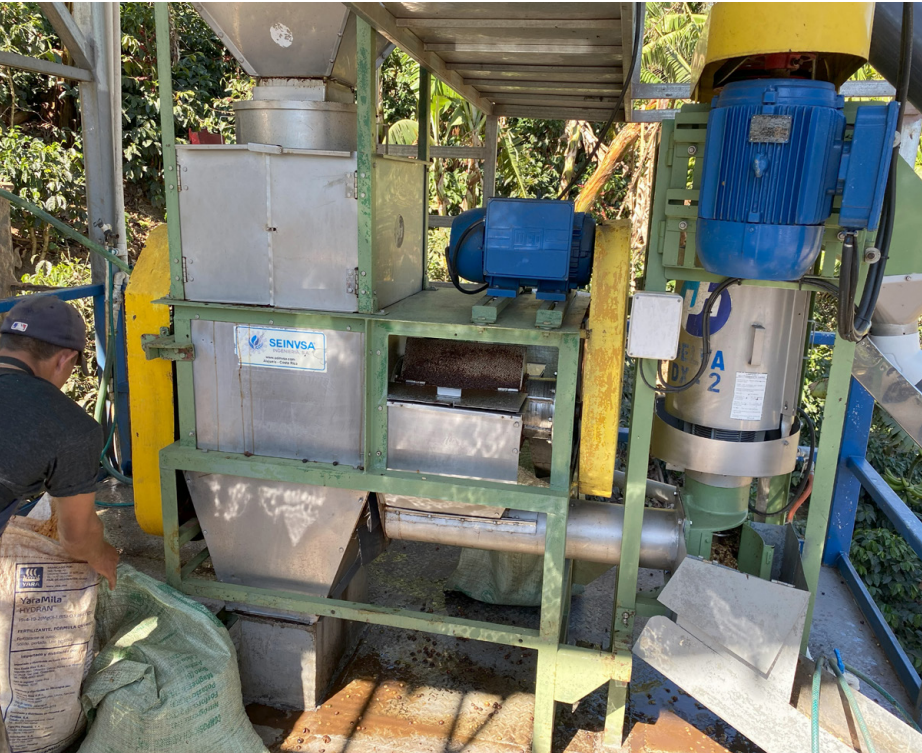
The main body of the pulper machine and a worker sorting rejects for a second run.
