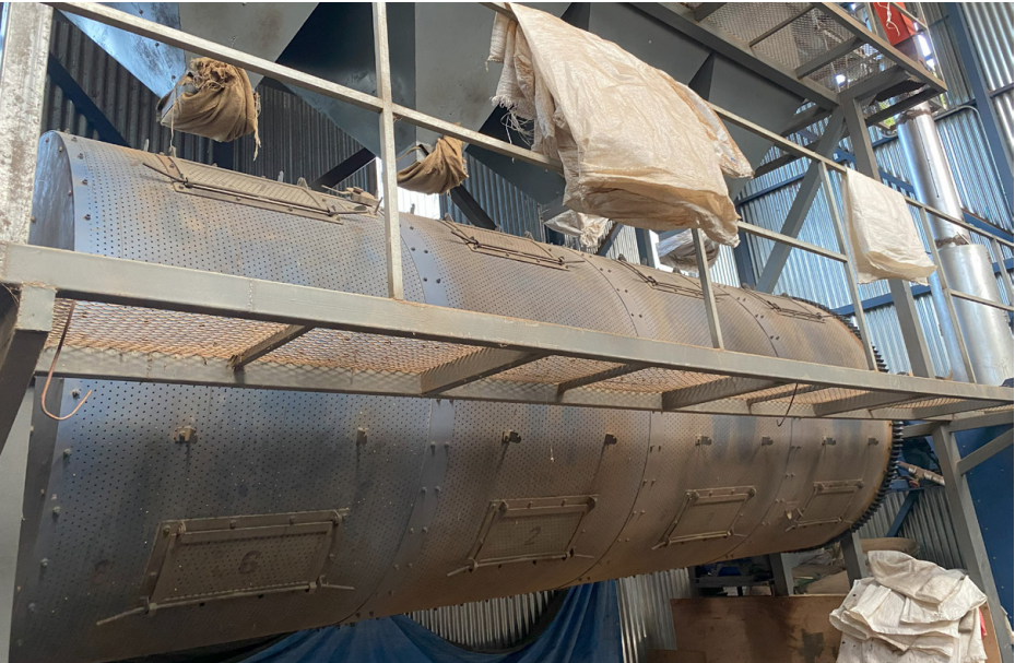
Mechanical dryer with a walkway for sampling and numbered doors for each compartment.
