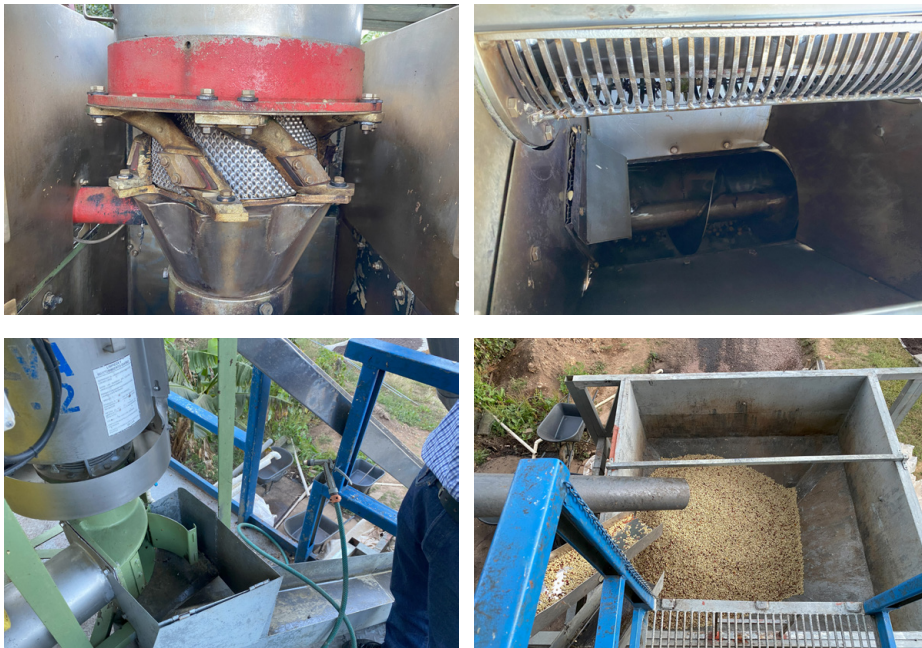
Pulper screen (top left), corkscrew (top right), exit shoot (bottom left), washed coffee (bottom right).
