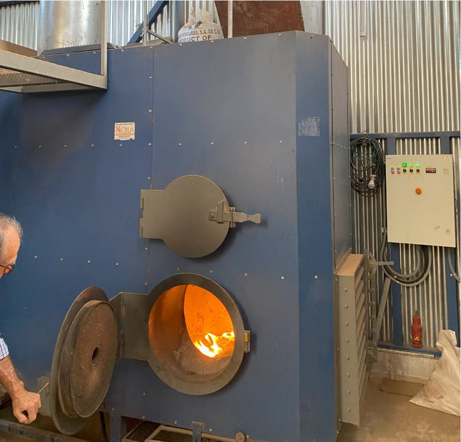
The furnace, kept at constant temperature, to dry the coffee in a controlled manner.
